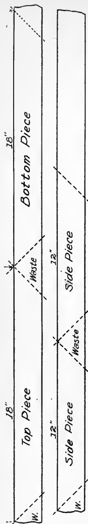
Fig. 1. Strips of Molding
